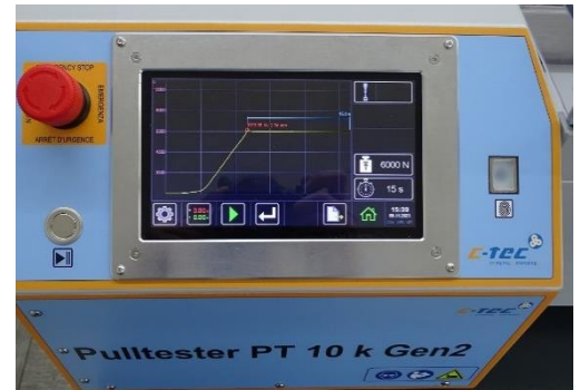
Display of the measurement curve in real time with zoom function
